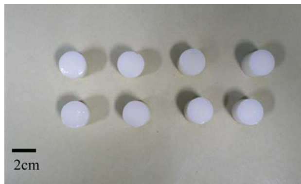
Fig. 5 Samples for mechanical property and in vitro degradation tests
